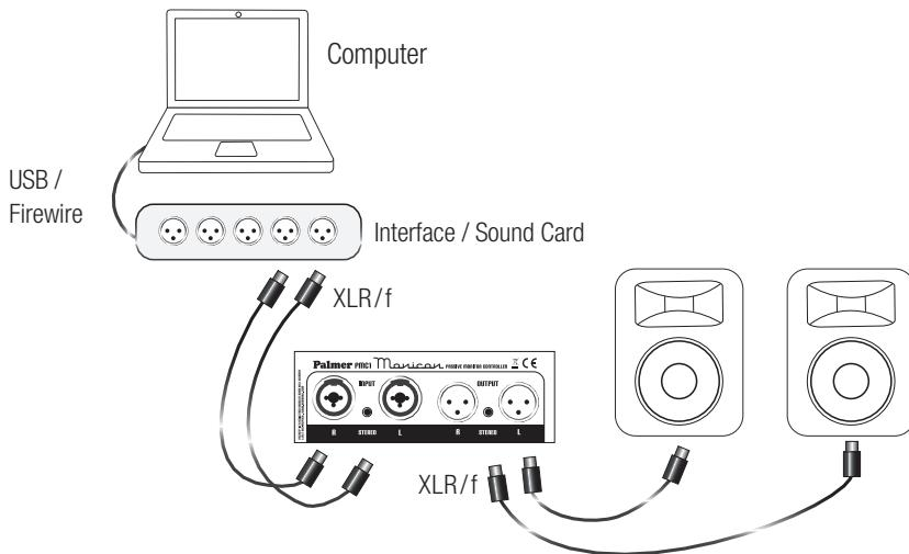
If your audio interface provides XLR or 6.35 mm TRS outputs use high quality shielded patch or microphone cables for balanced connection to the Monicon's L/R combo inputs.
