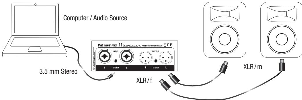
Use a 3.5 mm male to male stereo cable to connect the standard 3.5 mm line or headphone out of your desktop or laptop to the Monicon's 3.5 mm input.
