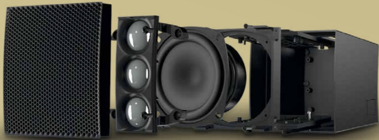
LD Systems' WaveAhead® technology places a vertical tweeter array in front of a high-performance full range transducer. This proprietary design reduces reflections from ceilings and floors resulting in clear, consistent coverage.
